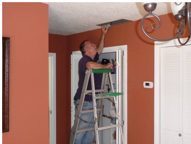
Figure 13. Air temperature and RH measurements were taken at House H51 using a Vaisala HM34 probe.
