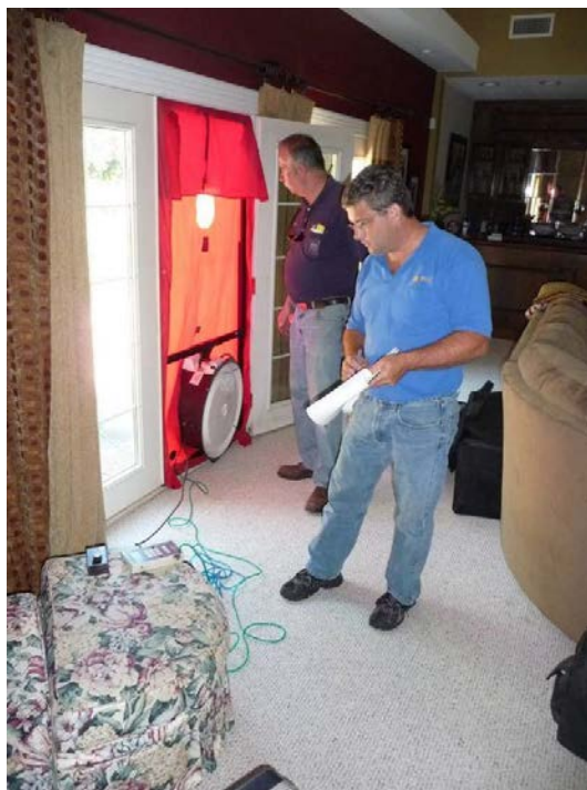
Figure 10. A baseline house pressure measurement is taken at the start of a blower door test at House H50.
