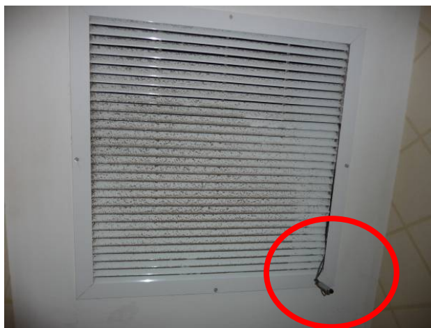
Figure 28. Temperature and RH measurement of first-floor return air at House H36M
