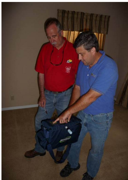
Figure 11. A house air infiltration test (with AHUs operating continuously) is performed at House H52 using a Bacharach specific gas analyzer.
