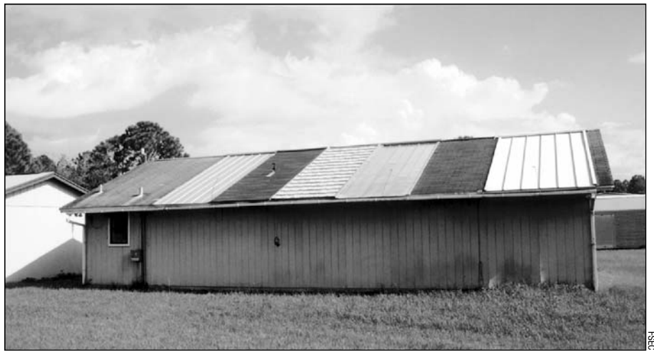
FSEC's Flexible Roof Facility allows side-by-side testing of different roof configurations.
