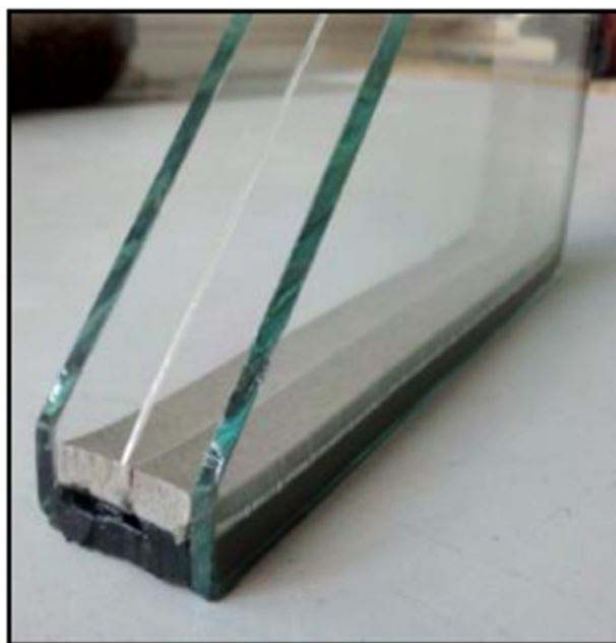
Figure 3. Thin Triple-Pane Window Design showing the Thin Glass Center that Floats on the Spacer and Low-E Coatings on the Second and Fifth Surfaces (Hart and Selkowitz 2018)
