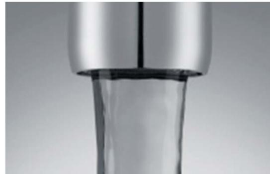
**Spray** When the flow rate is too low to produce an aerated or laminar stream, a spray device is used to produce a miniature shower pattern to provide full coverage of the hands during washing. Sprays are recommended for use in public lavatories.
