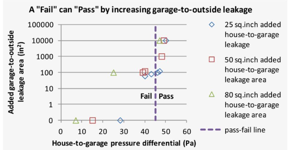
Test results showing the inadequacy of house-to-garage pressure differential as a single criterion for house-to-garage airtightness.
