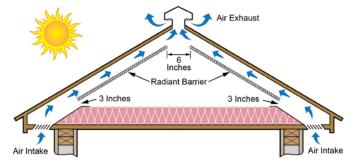
To prevent moisture problems when installing a radiant barrier, leave adequate gaps for air flow above, below, and behind the barrier material.
