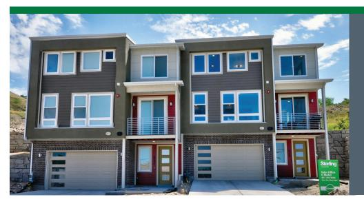
"At Sterling on Capitol Hill, we wanted to incorporate a modern look but we didn't want to use a flat TPO roof," said Mora, due to issues they've seen with flat roofs leaking in their high-snow-load location. On these homes, the eave of the simple gable roof runs parallel to the front and back elevation. Because the pitch is so low, the roof appears to be flat from the front and rear street level.
