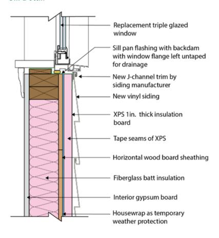
For the head and sill details, the view is from the side and the interior of the home is to the left of the wall. For the jamb detail, the view is from the top and the interior of the home is below the wall.
