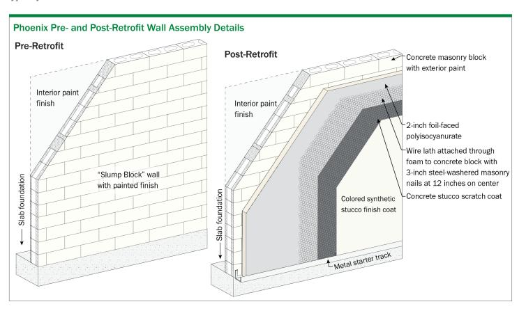
for using polyiso instead of EPS and for the 3-inch fasteners, steel washers, and the J weep flashing, which had to be custom made.
