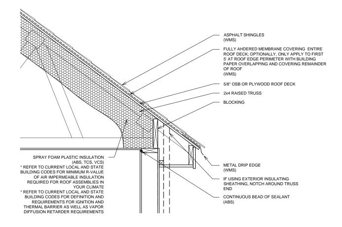
UNVENTED ATTIC 2x4 RAISED TRUSS - INSULATION BELOW ROOF DECK
