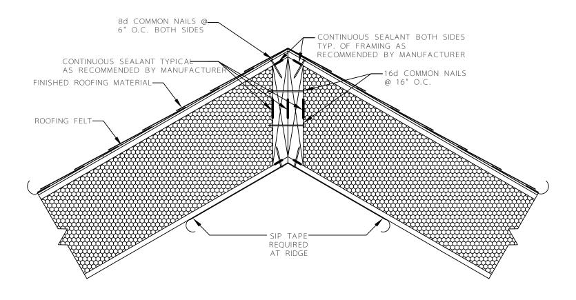
ROOF-TO-ROOF PANEL CONNECTIONS
