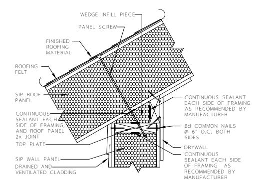
ROOF-TO-WALL PANEL CONNECTIONS WEDGE INFILL PIECE
