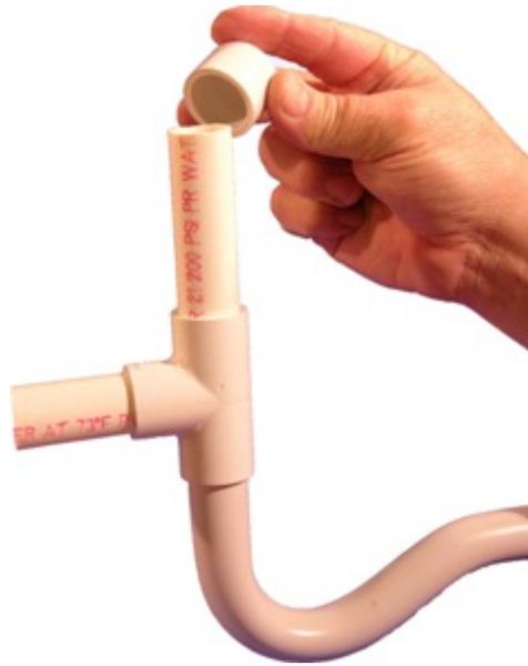
**Figure 4.** The drain pipe should include a trap and a clean-out with a removable cap. (Image Source: [KC Hart and Company](#))
