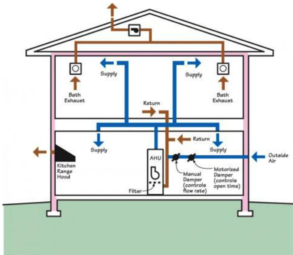
**Figure 1** – A fresh air inlet is ducted to the return side of the home's central air handler; a motorized damper and electronic controls help balance the flow of fresh incoming air with controlled exhaust to meet ventilation requirements (Source: [Local Exhaust and Whole House Ventilation Strategies](#))
