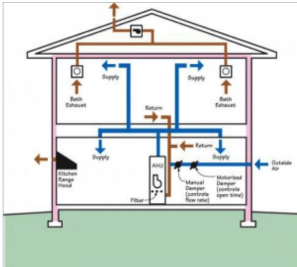
A fresh air inlet is ducted to the return side of the home's central air handler; a motorized damper and electronic controls help balance the flow of fresh incoming air with controlled exhaust to meet ventilation requirements
