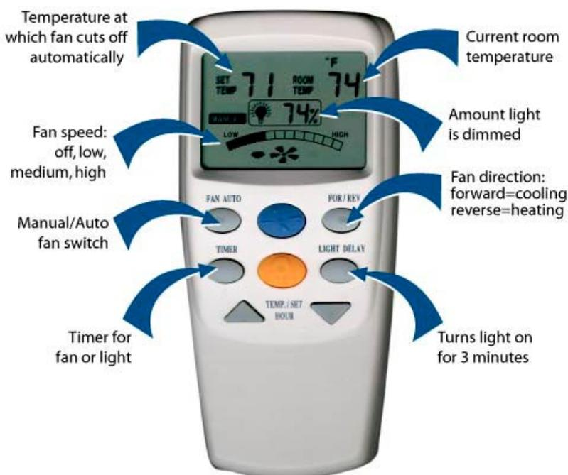
Figure 1. Remote control for a ceiling fan.
