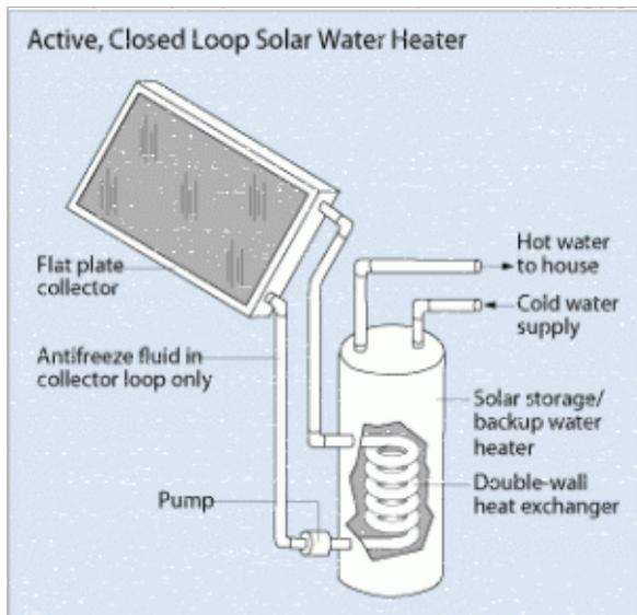
Install an indirect (anti-freeze) active solar thermal system.
