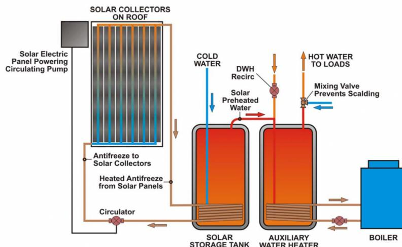
Figure 1. Two-tank indirect solar system.
