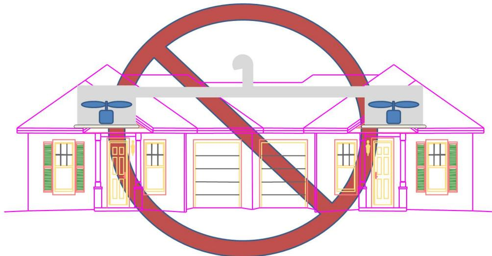
**Figure 1** - Exhaust fans in separate dwelling units should not share a common exhaust.
