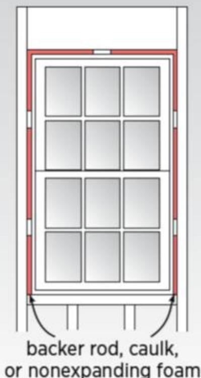
**Figure 1** - Air seal door and window rough openings with backer rod, caulk, or nonexpanding foam. (Image courtesy of PNNL)
