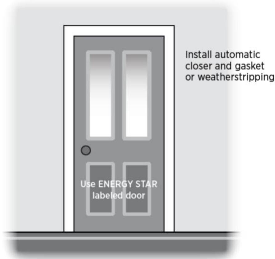
**Figure 2** - Install an ENERGY STAR-labeled door with an automatic closer. Weather strip the door frame. (Image courtesy of PNNL)
