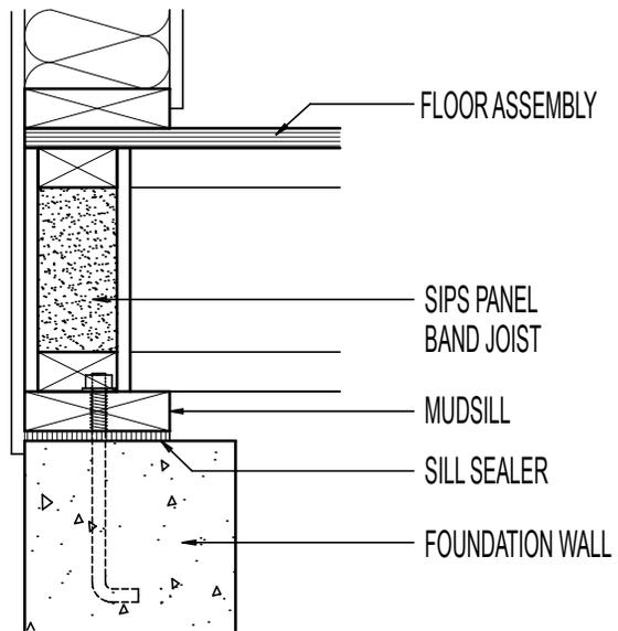
STRUCTURED INSULATED PANELS (SIPS) AS BAND JOIST
