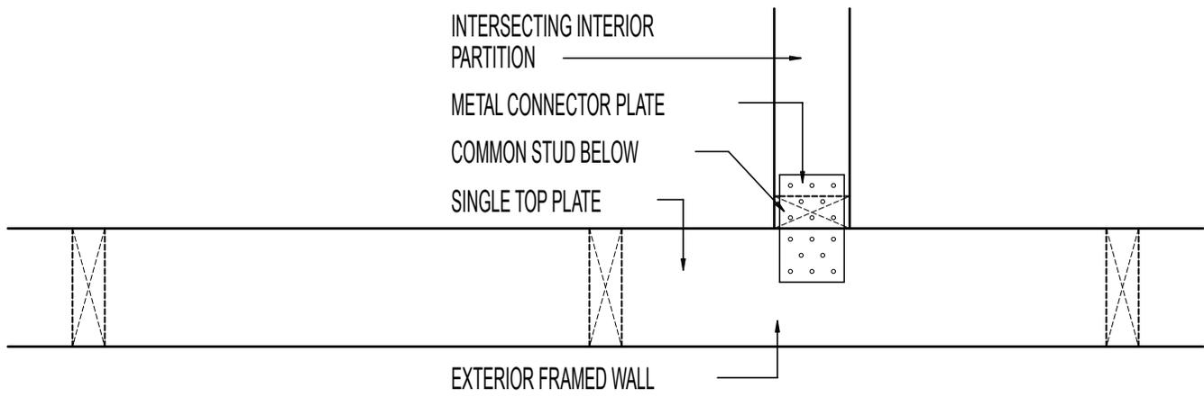
TOP OF INTERIOR INTERSECTING WALL WITH METAL PLATE
