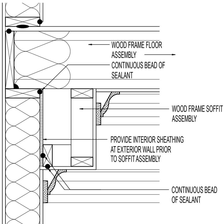
AIR SEAL AT BUILT-OUT SOFFIT
