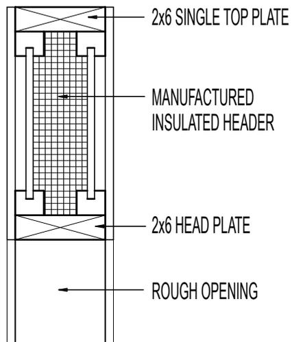
MANUFACTURED INSULATED HEADER
