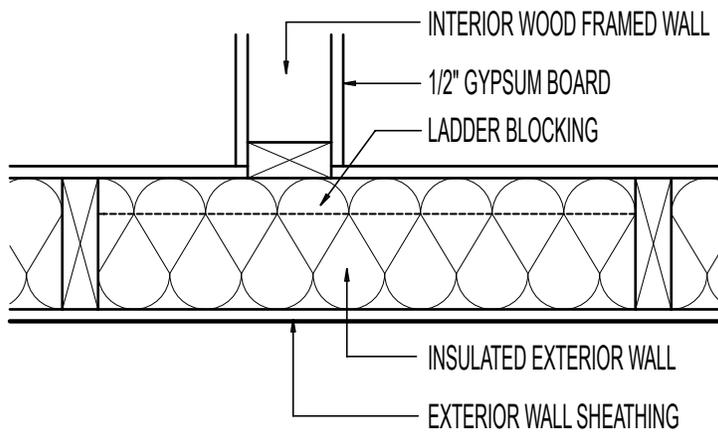
INTERIOR INTERSECTING WALL WITH LADDER BLOCKING
