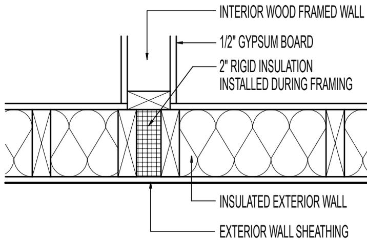
INTERIOR INTERSECTING WALL WITH 2 STUDS AND RIGID INSULATION
