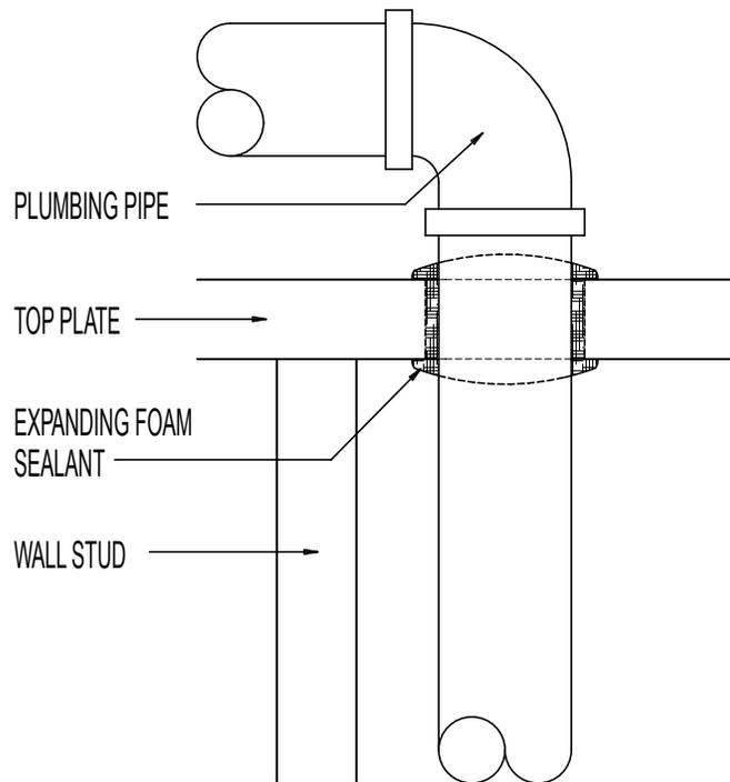
AIR SEAL AT TOP PLATE PIPE PENETRATION
